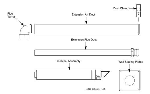
Fig. 20 Flue Components
