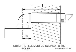
Fig. 21 Flue length - rear
