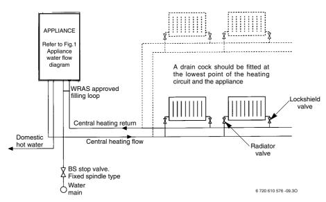
Fig. 5 Sealed primary water system
