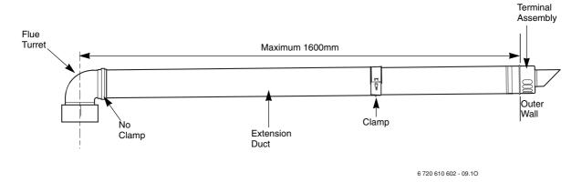
Fig. 18 Flue with One Extension
