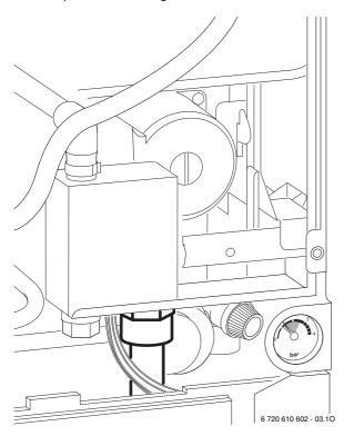
Fig. 12 Position of the condensate drain
