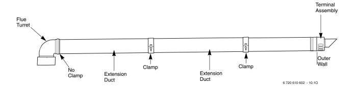
Fig. 19 Flue with Extensions
