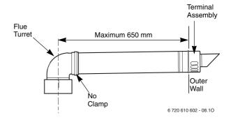
Fig. 17 Standard Flue
