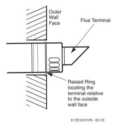
Fig. 23 Flue terminal position
